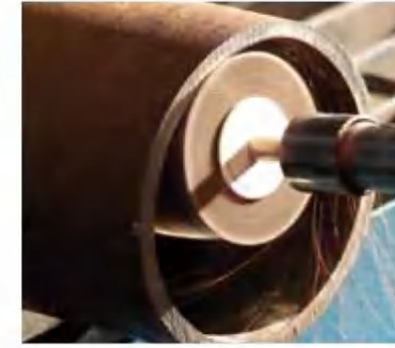
Removing burrs from the inside diameter (ID) of a cut tube.
